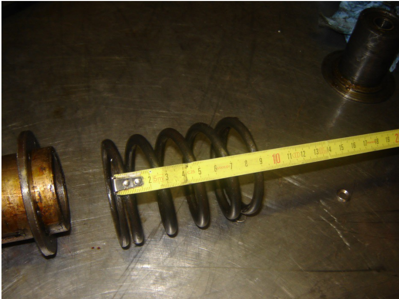
Peugeot bebe 1913 Inner clutch spring
